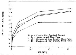
Fig. 1 — Compressive strength of wet-mix shotcrete.
