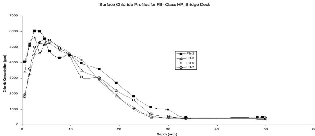
**Figure 2. Typical In-service Chloride Penetration Profiles**
