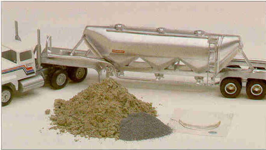
The second step in batching HP concrete is to slowly add the cement with microsilica batched on top. Finish up with high-range water reduction chemicals and the remainder of the batch water. Photo courtesy of Elkem Materials. Photo by John Wee
