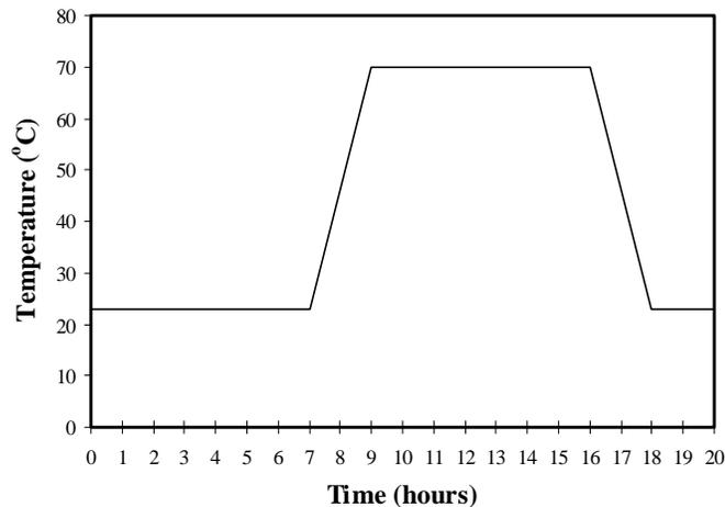
*Figure 1 - 18-hour steam curing cycle*
