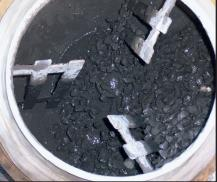
and some of the water. Never batch the silica fume alone or first into the mixer. Mix these materials for  $1\frac{1}{2}$  minutes.
