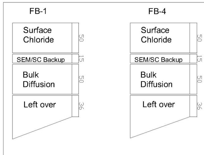
**Figure 1. Typical arrangement of saw cuts on cores for testing (depths shown in mm)** (Note: SEM/SC backup slices were reserved for microscopy, but were not tested)
